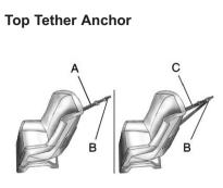
A top tether (A, C) anchors the top of the child restraint to the vehicle. A top tether anchor is built into the vehicle. The top tether attachment (B) on the child restraint connects to the top tether anchor in the vehicle in order to reduce the forward movement and rotation of the child restraint during driving or in a crash. Your child restraint may have a single tether (A) or a dual tether (C). Either will have a single attachment (B) to secure the top tether to the anchor.
